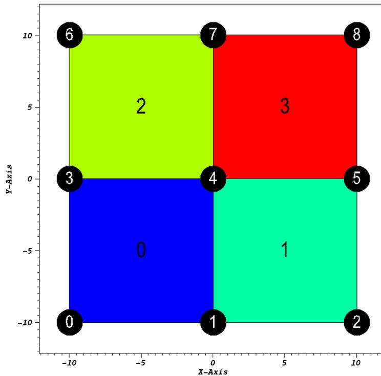
Fig. 6: Pseudocolor plot of basic (mesh type 'quads')
